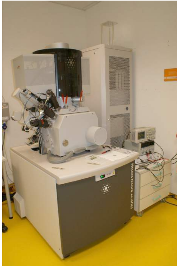
Figure 3.8: FEI Helios 600i FIB tool for nano-manipulation of samples.
